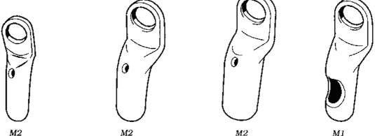
BAC cable lugs are specially manufactured in the intended material for pin brazing. Consult the table of recommendations on the choice of a suitable cable lug. The lugs are made in two different types. M1 is pin brazed to the cable. M2 is crimped to the cable.
